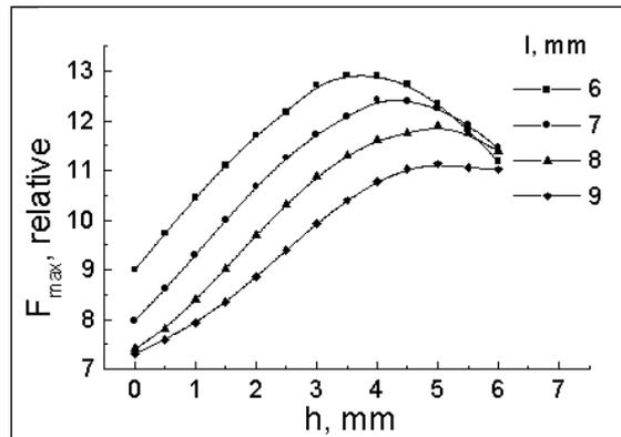
Figure 11: Maximal beam pattern amplitude  $F = F(h, l)$ , where  $h$  and  $l$  are distance between array levels and radiator spacing correspondently.
