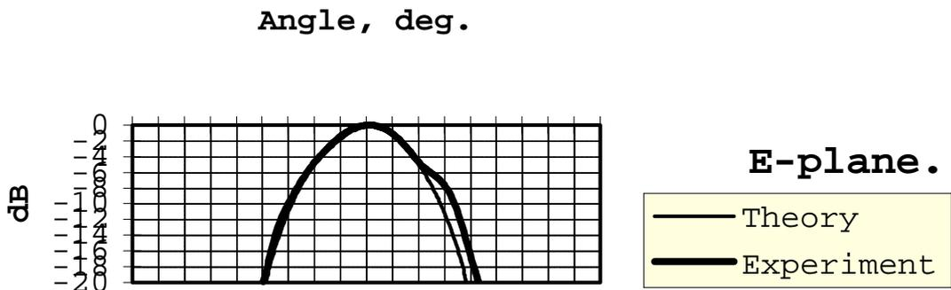
Figure 6: Power beam pattern of a microstrip radiator (5.9x3.4 mm) in 8-element array in E and H-planes
