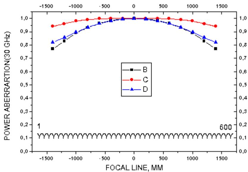
Figure 9: RATAN-600 power aberration curves along the focal plane
