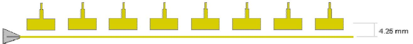
Figure 5: The loaded microstrip line for communal channel calibration
