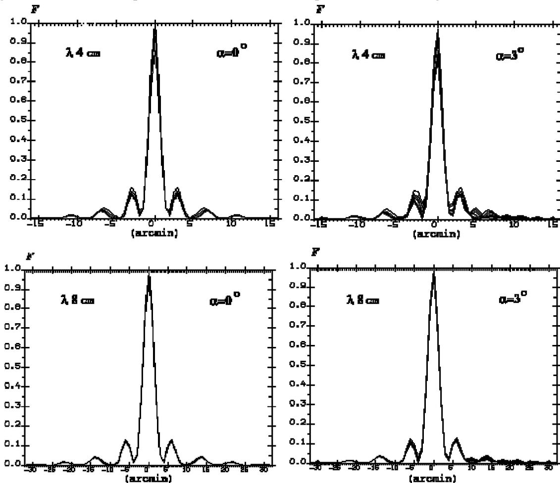
Figure 12: RATAN-600 power beam patterns in Radio-Schmidt mode for different elevation angles and half an hour cosmic source tracking
