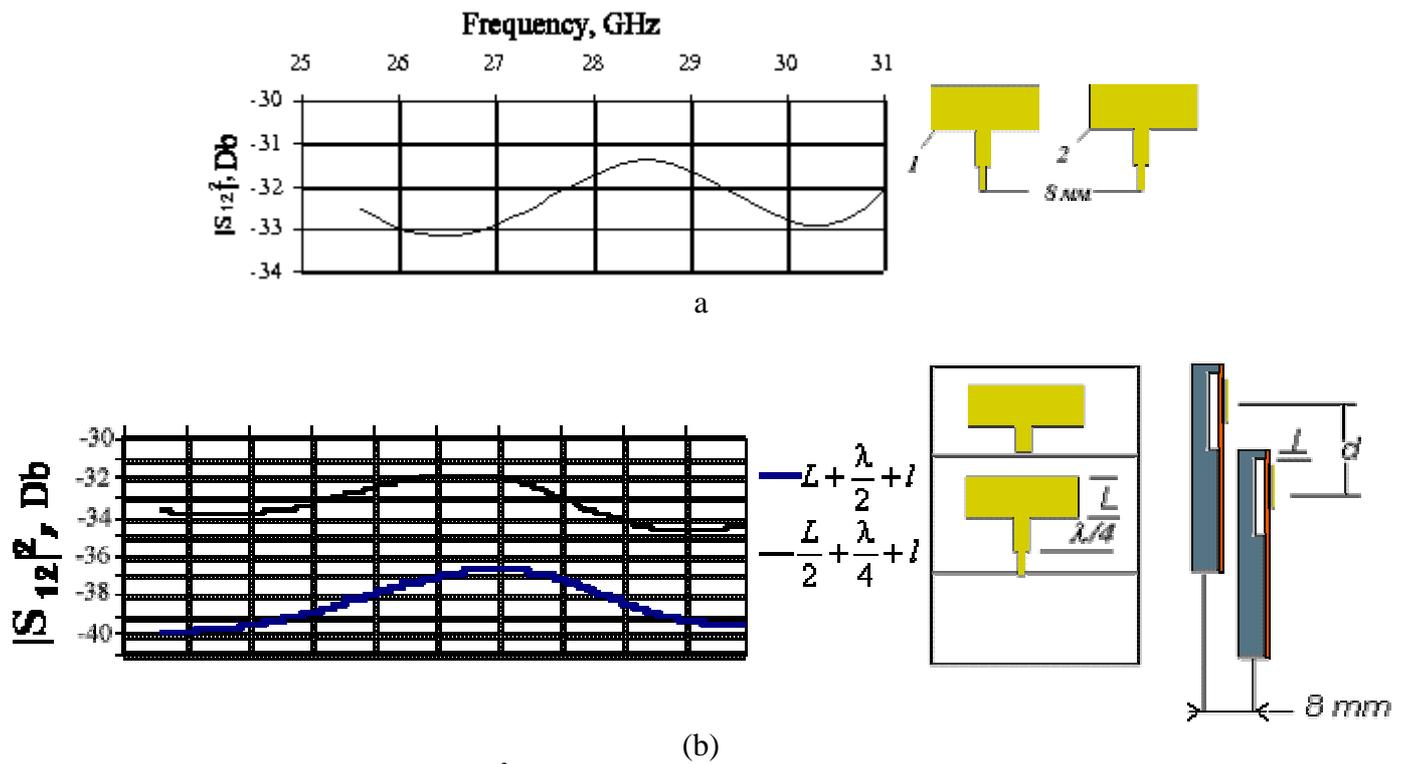
Figure 2: Mutual coupling  $|S_{12}|^2$  for microstrip radiators (5.9x3.4) mm of one array level in H-plane (a), mutual coupling  $|S_{12}|^2$  for radiators of different array levels in E-plane(b).
