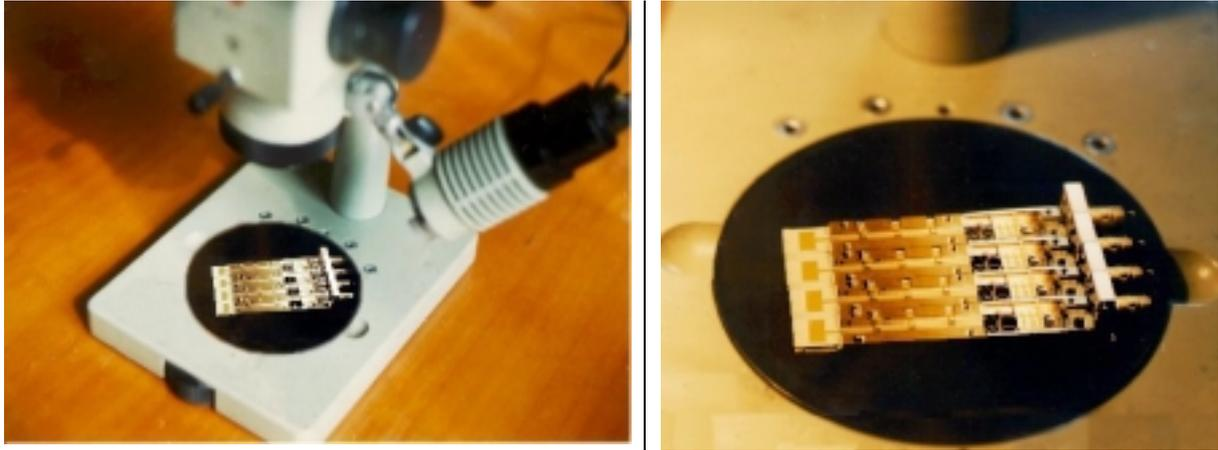
Figure 4: 4-element sub-array prototype at 26-30 GHz.
