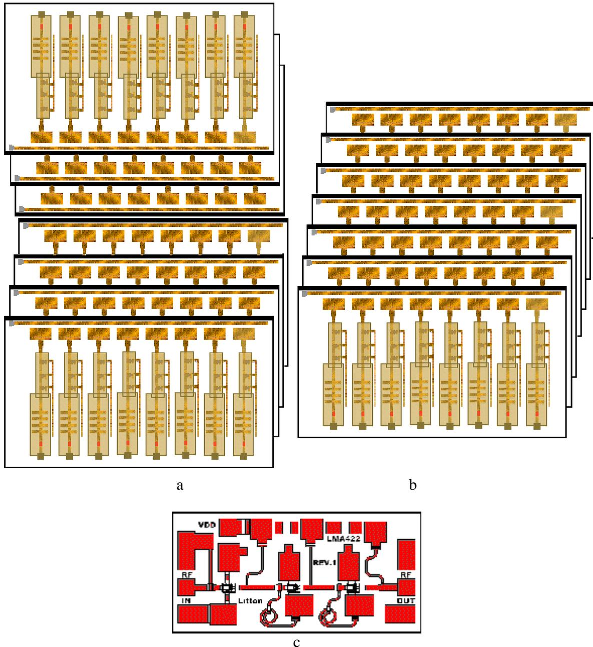
Figure 1. "Terraced" 7x8 element MMIC array architecture (a, b), MMIC amplifier LMA422 of Litton SSD(c).
