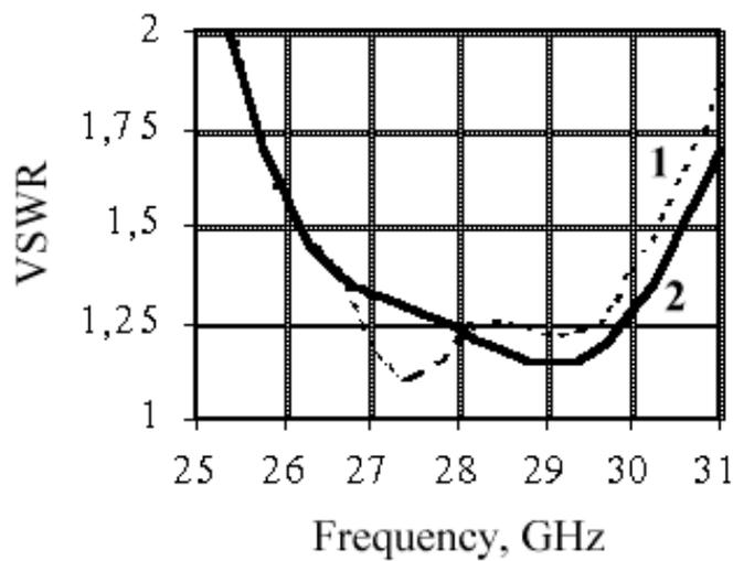
Figure 3: VSWR of microstrip radiator for one (1) and three (2) dimensional arrays.
